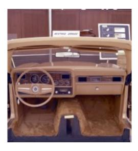
1974: With the launch of the all-new second-generation Mustang II, design took a new, contemporary direction. The three-spoke wheel was replaced with a leather-wrapped two-spoke wheel. Mustang II introduced available power rack-and-pinion steering — allowing cars equipped with that feature to have a smaller 15-inch wheel as opposed to the standard 16-inch one.
