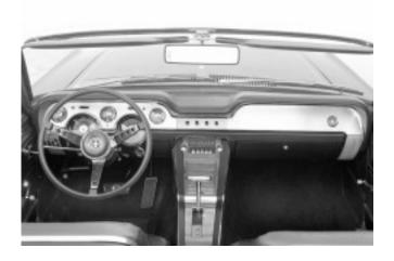
1967: As Mustang matured, new features were added to make it more functional and more convenient for enthusiast buyers. A tiltaway wheel with seven adjustments was available. This allowed drivers to choose the steering position that fit their preference, while also improving vehicle entry and exit without sacrificing looks or practicality. A new faster ratio (20.3:1) power steering system became available in 1967, making turn-in quicker for a sportier feel.
