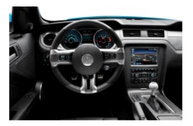
2013: In further refinement of the Mustang steering wheel as the incar tech control center, the wheel was revised to include a four-way control button, plus an "OK" button for instrument cluster screen control. Boss 302 and Shelby GT500 Mustangs got a race-inspired Alcantara-wrapped steering wheel.
