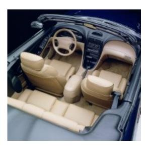
1994: The launch of the fourth-generation Mustang included a nod to the original 1964 pony car, with a twin cockpit layout and sculpted modern styling for the steering wheel and airbag. Various buttons became easier to use, while allowing for the driver to keep eyes on the road and hands on the wheel. Horn buttons were replaced with a hinged airbag cover, acting as horn control at the wheel's center.
