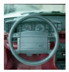
1990: Mustang received its first airbag as standard equipment. Because the airbag was located in the center of the steering wheel, the horn was moved from the center to two spokemounted buttons, easily accessible by the natural position of the driver's thumbs. Cruise control buttons were also placed in a more ergonomic position.
