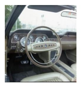
1968: Safety became a priority, and a collapsible steering column was added to Mustang to aid in reducing the possibility of injury in a crash. To bolster this feature, the redesigned two-spoke steering wheel featured a larger, cushioned center section. The center hub horn control was replaced with the small, metal half-circle on the bottom half.
