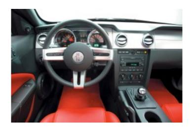
2005: Based on the 1965-1967 Mustang design, this three-spoke wheel appeared on the fifth-generation Mustang. This wheel was available with standard urethane spokes, or optional aluminum spokes with the interior upgrade package. Unlike the steering wheels it was based on, this rim came wrapped in leather.
