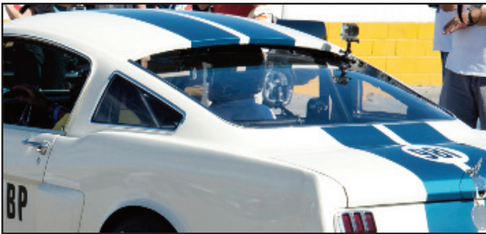
The shape of the plexiglass rear window was reconfigured to eliminate the pronounced “break” in its profile. The space at the top edge is only an inch and a half (the original windows’ space was closer to three inches); the smaller space is intended to make the cockpit air exit more efficiently. The window opening’s lip was also trimmed off.
