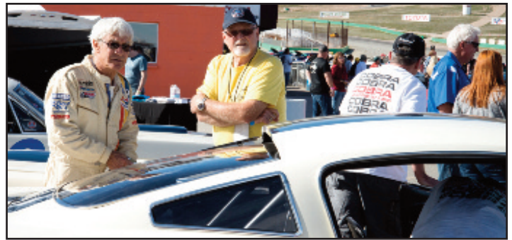
The shape of the plexiglass rear window was reconfigured to eliminate the pronounced “break” in its profile. The space at the top edge is only an inch and a half (the original windows’ space was closer to three inches); the smaller space is intended to make the cockpit air exit more efficiently. The window opening’s lip was also trimmed off.
