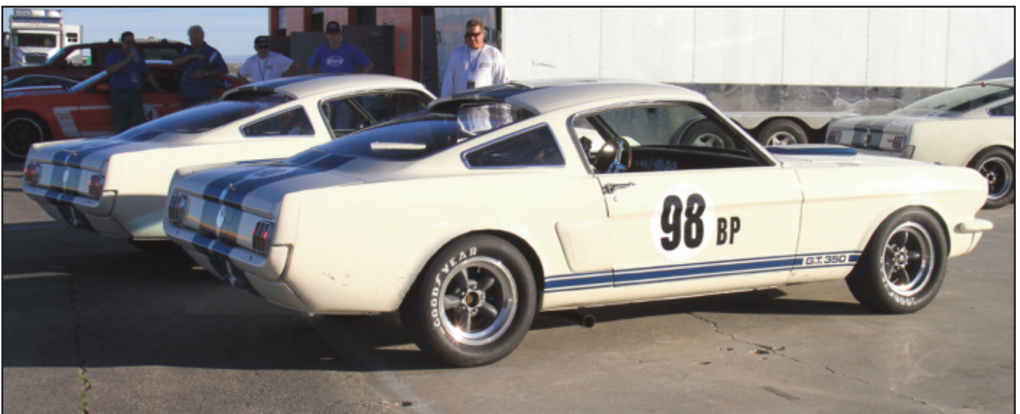
Since Jim Marietta started with 1966 Mustangs the decision was made to use '66 GT350 rear quarter windows. Aluminum window frames and plexiglass side windows were also eliminated, mostly to be able to meet the February 14th deadline. Besides, these windows are never used, anyway.
