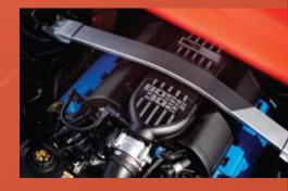
"Runners-in-the-box" intake plenum enhances airflow for charges to the redline
