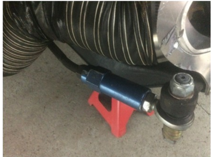
"Slightly" bent tie rod.
