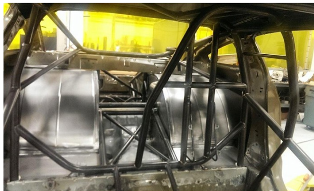
Chris Holbrook's Super Stock Mustang roll cage and tubbed rear wheelwells
