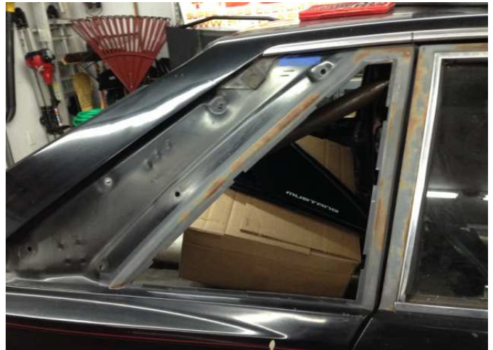
Early Fox small window car with window removed, & new hole marked (tape area), & molding marked to be cut off.
