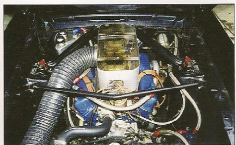
The business end of the Shelby Mustangs is representative of the mid-season state-of-the-art induction system. The air box is an adaptation of the GT40 ram air system. Clearly visible are the export bracing from the shock towers and the Monte Carlo bar at the front of the engine. (Photo Courtesy Phil Jacobs Collection)
