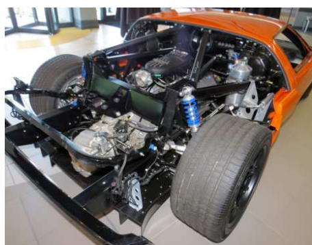
Jim Dunham's GT racer proposal with a BOSS 302 Modular engine
