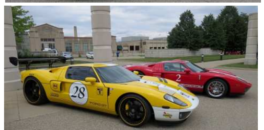
Bailey's GT, nicknamed "Mellow Yellow", one of the more heavily modified GTs, with twin turbos, aftermarket wheels, graphics and rear wing
