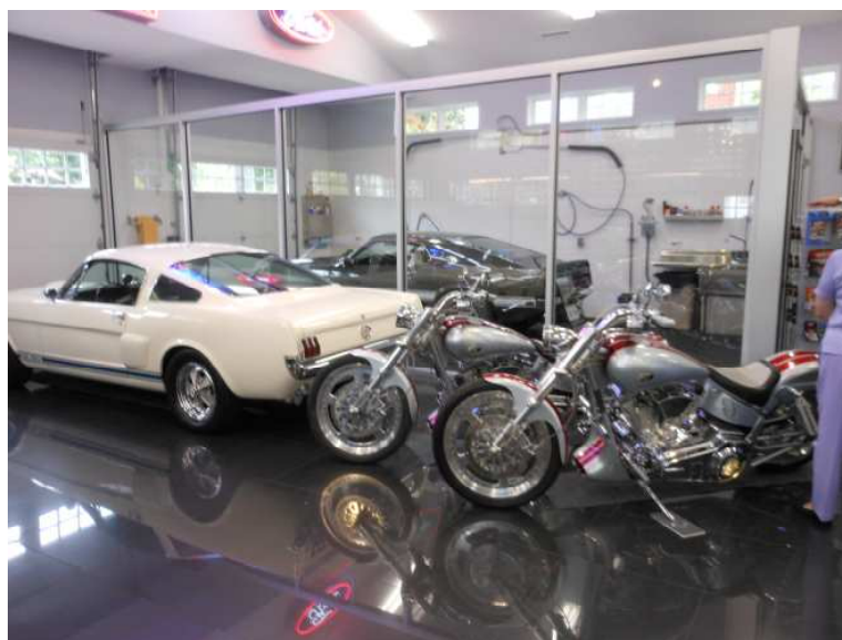
Two Shelby Series I Titan motorcycles that are powered by a 112 cubic inch, 115 HP engine. The Shelby company offered buyers of the Series I the chance to purchase a Titan Shelby with a VIN matching their car's.
