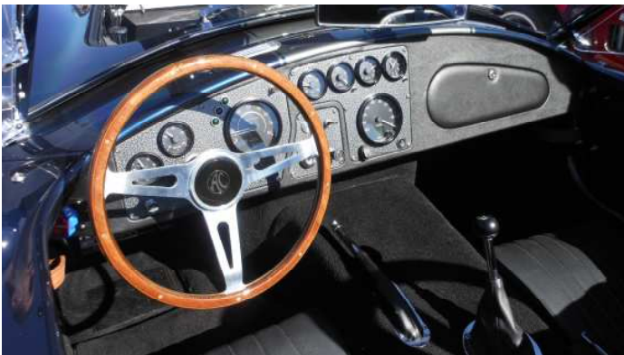
Tip's dash is manufactured by Casey Design Products. It is a modular design that allows easy access to the wire harnesses (less time on your back). A Casey modular dash is also available for the Daytona Coupe. Also, notice Tip's convenient location of the emergency brake handle, on the left side of the trans tunnel.
