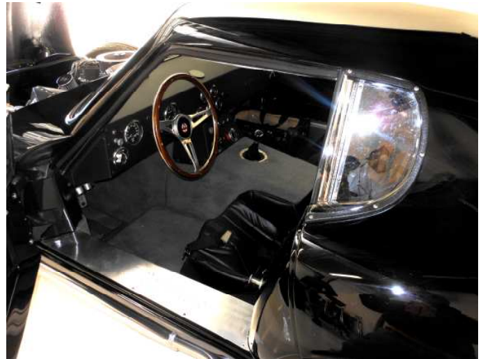
Garry's interior photo shows the Russ Thompson aluminum door sill plate and the hinged rear quarter window, behind the curved plexiglass air scoop.
