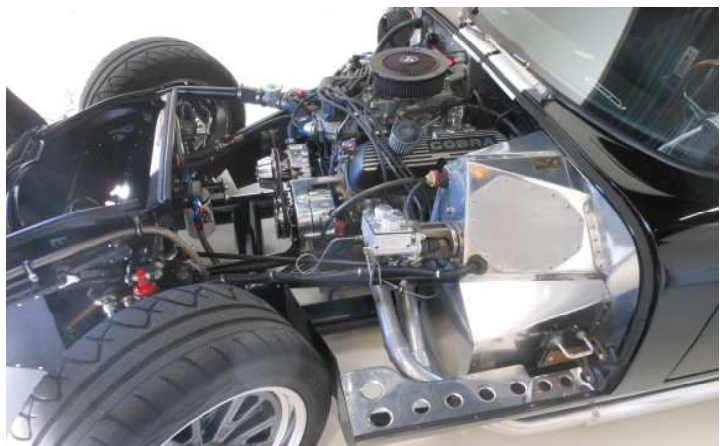
Garry's beautiful engine compartment contains a 422 ci, 351W engine.
