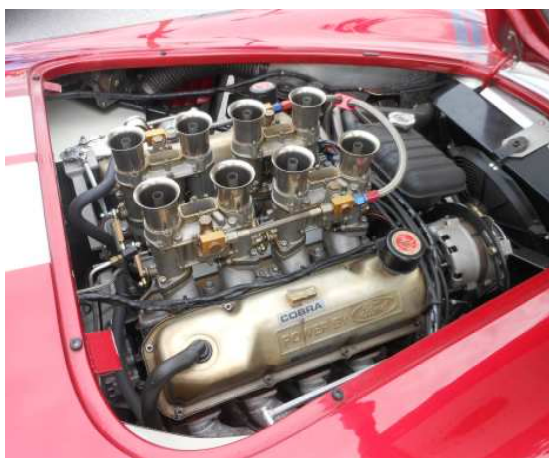
Below Left: Jeff Burgy's BOSS 351 engine is slightly bored and stroked, and features a 4-bolt main Australian block, Carillo rods, solid lifter camshaft, Canton road-race oil pan, steel valve covers with extra breathers, all topped off with a set of 48IDA Weber downdraft carburetors. Very similar to what an original 289 FIA Cobra would run, except for a few additional cubic inches.
