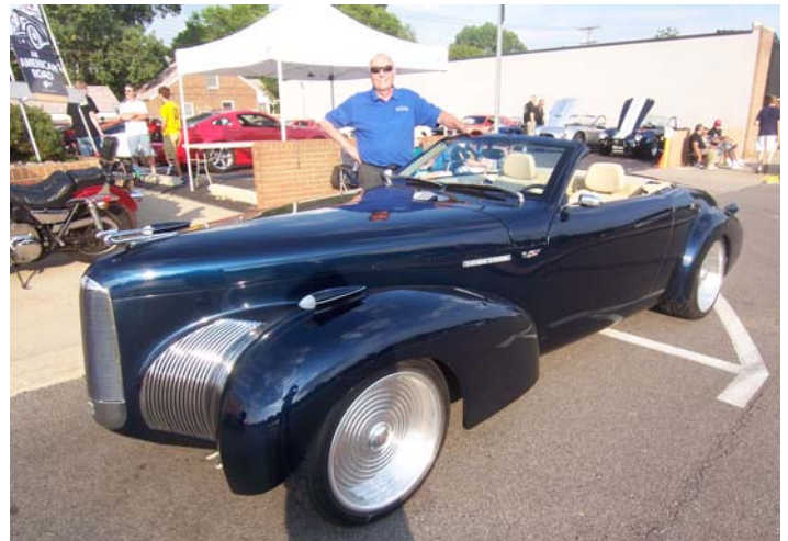
Steven D. Pasteiner, Steve's father, owns Advanced Automotive Technologies (AAT). AAT is a full house prototype company. They have the ability to build what they design. Steven brought a beautiful example of what they can design and build. It is a La Salle C-Hawk. Built on a custom frame while utilizing Corvette C4 suspension modules and a Cadillac CTS-V engine.
