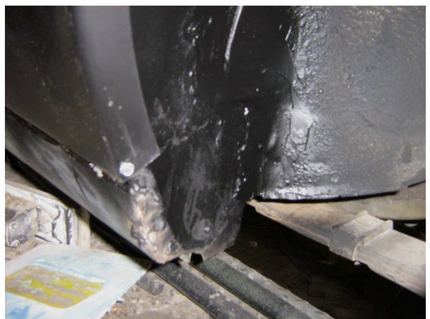
New quarter panel temporarily secured with a sheet metal screw at the rear wheel well opening.
