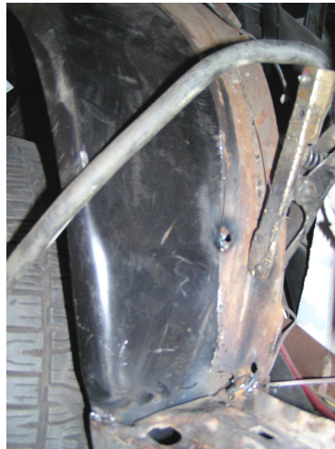
New outer wheel well lapped over old one and tack welded
