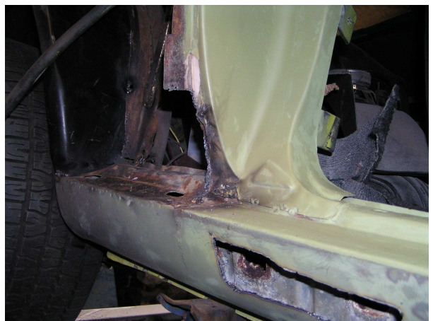
Area trimmed at rear door jamb. Notice the rocker panel needed a repair patch.
