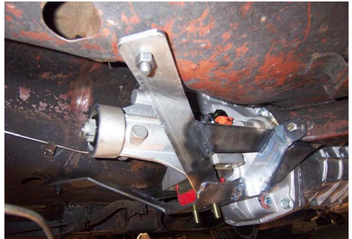
Transmission mount cross member was fabricated from 3/16" steel and designed to attach to the stock sub-frame location and holes drilled through each flange of the seat perches where they meet the floor. This picture was taken before the part was powder coated.
