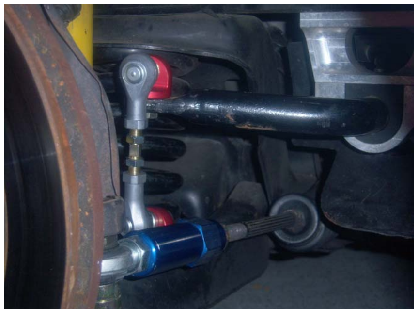
Adjustable sway bar endlink installed with the sway bar in proper set-up position.
