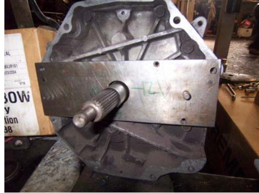
This is the plate developed to check the center of the bell housing
