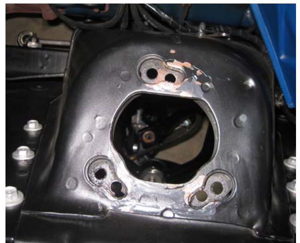
3 holes need to be drilled into the stock upper spring seat on 67-70 cars, no holes are required for 65-66 cars.
