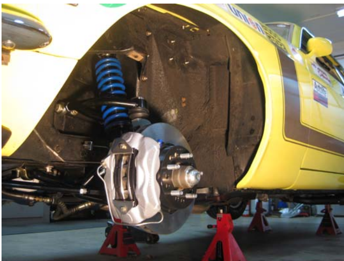
Street or Track Bilstein Coilover System completely installed. All show in the engine bay, all go underneath!
