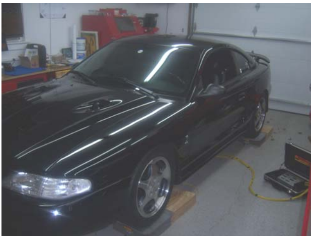
Each wheel is on a flat weight scale which are connected to the readout display unit
