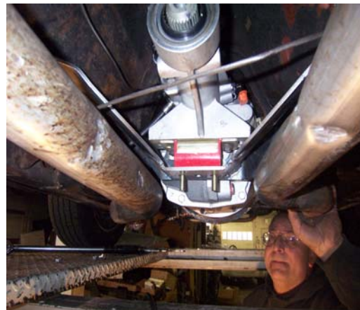
Transmission mount cross member was fabricated from 3/16" steel and designed to attach to the stock sub-frame location and holes drilled through each flange of the seat perches where they meet the floor. This picture was taken before the part was powder coated.
