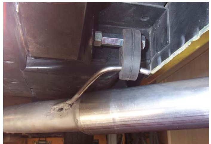
The hex threaded coupler is attached to the front eye bolt of the rear leaf spring. The rubber insulator hanger is attached to the other end of the hex threaded coupler.
