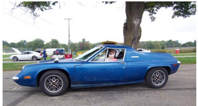
"Sam Doe's" 1972 Lotus Europa TC Special has a mid-engine rear-wheel drive layout and utilizes a Lotus "Big Valve" Twin Cam engine and weighs 1,400 pounds. The body is very thin fiberglass to help keep the weight low.
