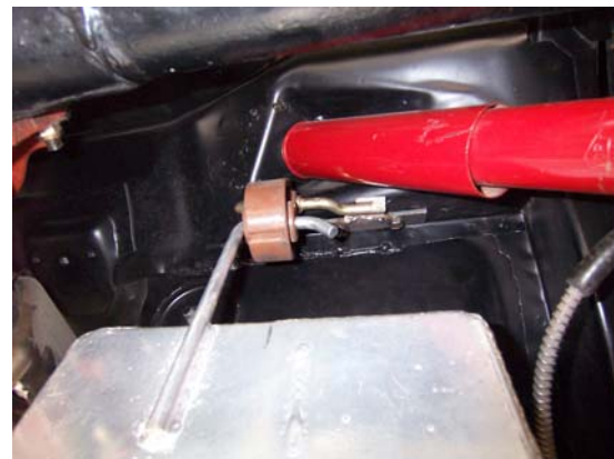
The muffler hanger I obtained from Walt Berti is located at the end of the muffler hanger rod and is welded to a plate I fabricated to utilize the existing floor pan mounting holes.
