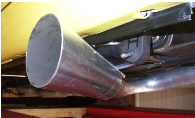
Exterior view of the hanger for the exit end of the J-pipe.
