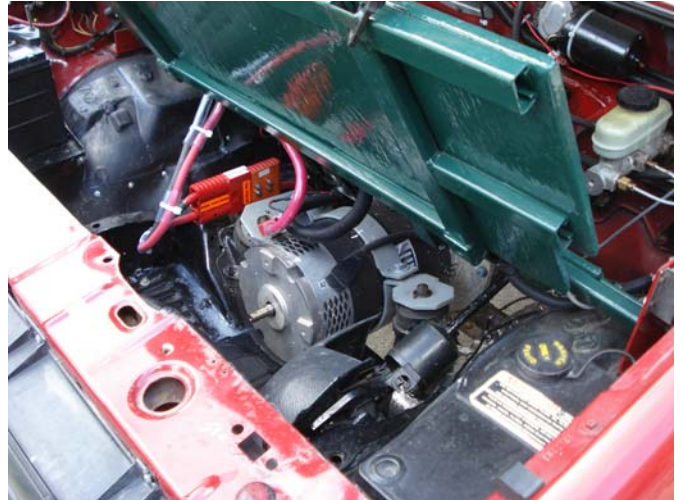
Electric components mounted on a hinged plywood panel allow access to the electric motor.
