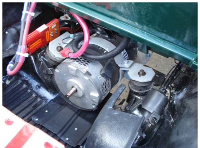
The electric motor is connected directly to the transmission.
