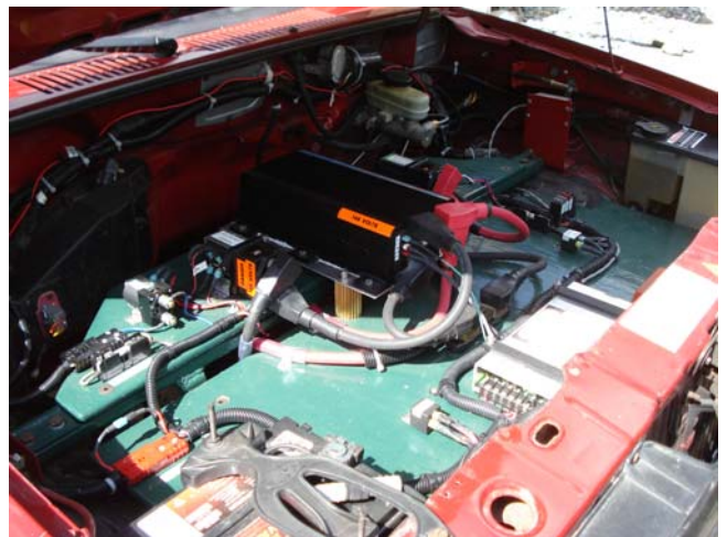
Electric components mounted on a hinged plywood panel under the hood.
