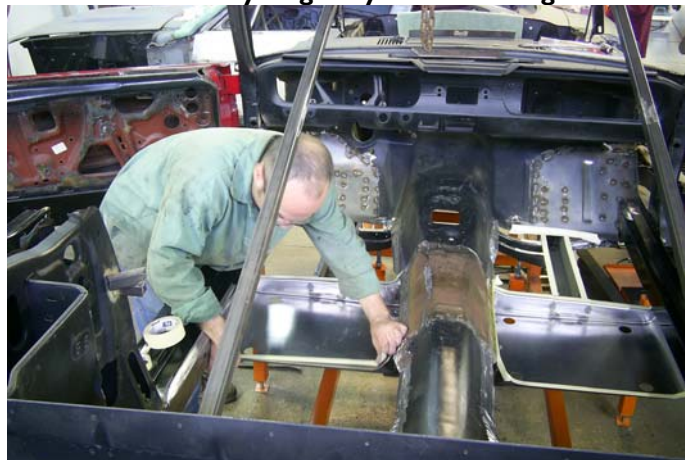
The fixtures under this Mustang were designed by Mroz to hold the car straight and square much as Ford did when they originally built Mustangs.
