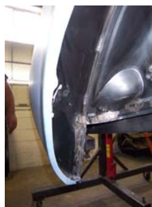
Left: Evidence of expert metal work where the rear quarter attaches to the wheel well.
