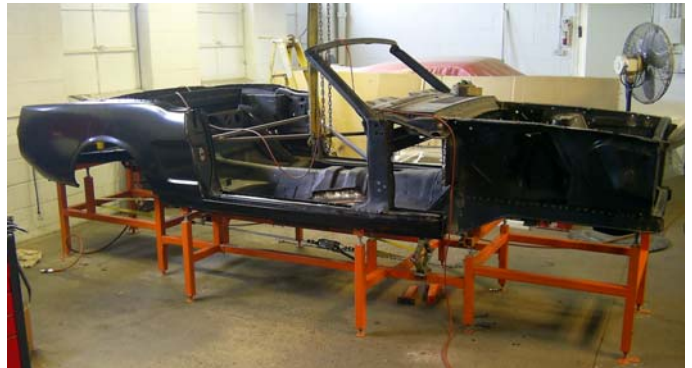
The fixtures under this Mustang were designed by Mroz to hold the car straight and square much as Ford did when they originally built Mustangs.
