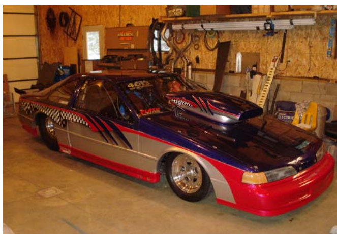
1993 Thunderbird body made up of steel roof and quarter panels, carbon fiber doors, front clip and hood with a fiberglass hood scoop.
