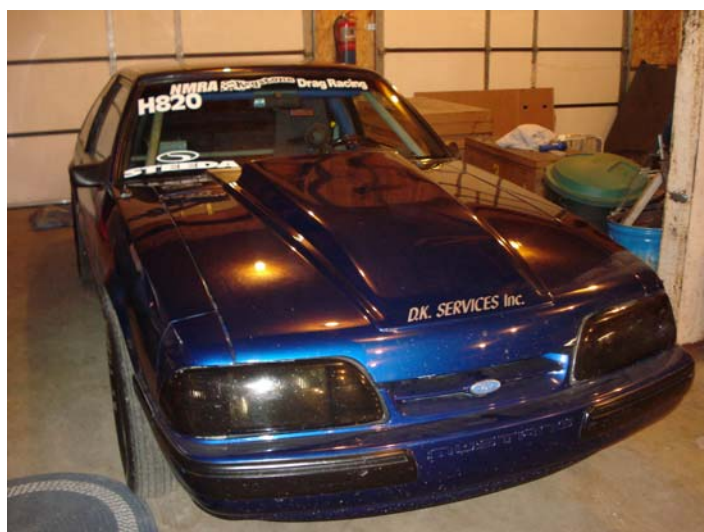
Dave Krzyzanski's 1988 Mustang has a 302 bored and stroked to 363 ci. His best 1/4 mile ET was 10.18 seconds and top speed of 131 MPH in this car.
