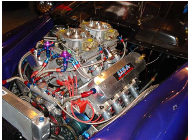
The engine has Chuck Nuytten carbs on it and puts out 1,150 horsepower. A nitrous boost adds 400 more ponies.
