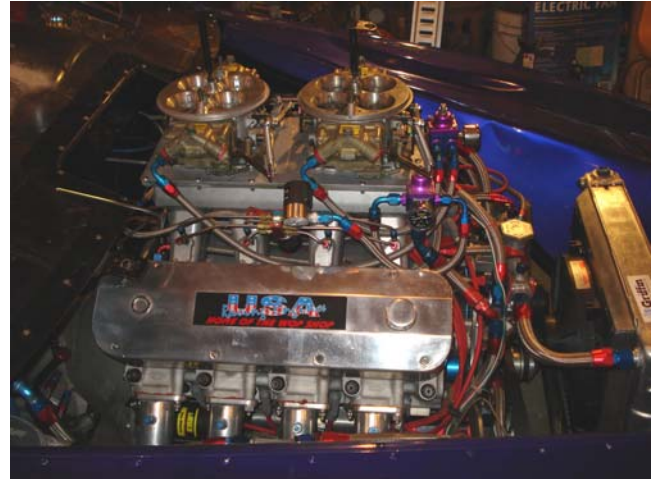
The steel SVO engine block, with aluminum heads, has 598 cubic inches.
