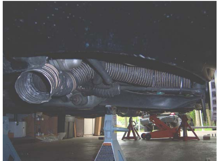
The entrance end of the 3" brake cooling hose is just below the air dam on the front fascia
