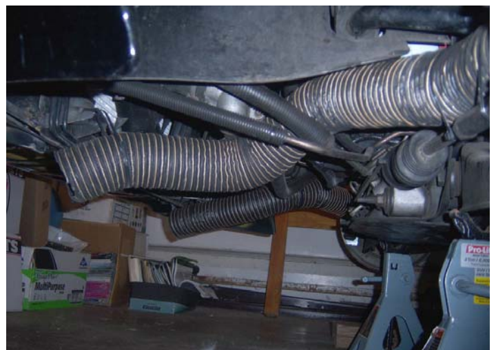
The entrance end of the 3" brake cooling hose is just below the air dam on the front fascia
