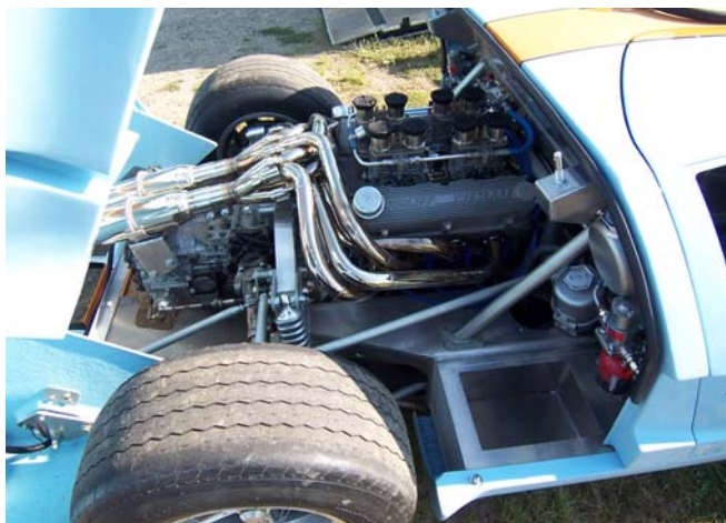
Rob Borruso's GT40 Mk I Chassis was designed to accommodate the Ford 289 engine and the ZF-2 five speed gear box.
