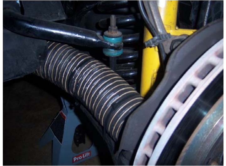
3" brake cool hose tie wrapped to the tie rod and exiting near brake dust shield
