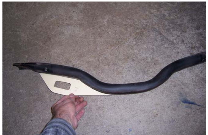
Steve checks the tie-down modification for proper fit, with a template before cutting them out of 3/16" thick steel.
