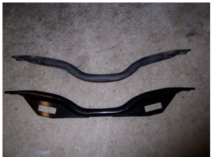
Comparison of stock (top) to modified cross-member with tie-downs (bottom).
