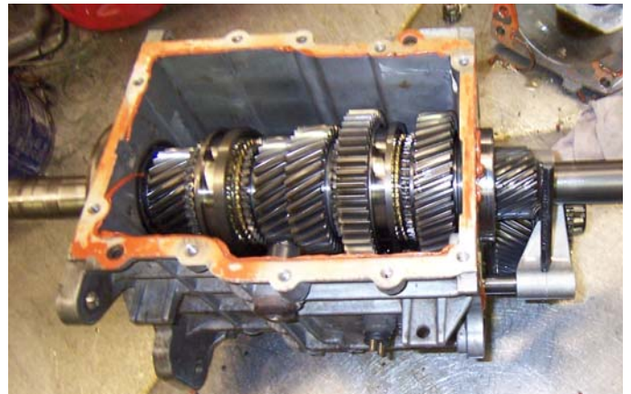
The transmission case inspection plate and rear housing have been removed exposing the out put shaft assembly and fifth gear assembly, outside the transmission case to the right.
