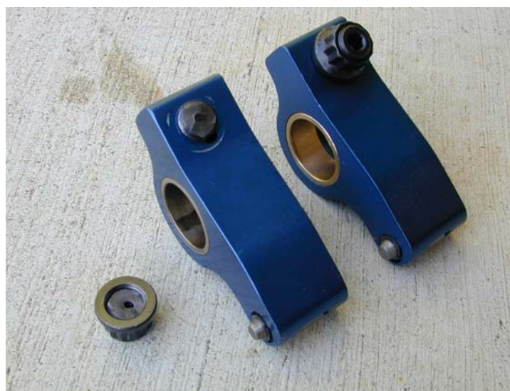
Precision Oil Pumps rocker arms have low-quality adjusters that snapped in two during hard driving.
