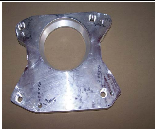
John Yarema fabricated this adaptor plate and made improvements based on a bad experience with an after market plate.
