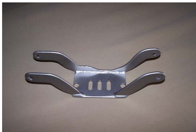
John Yarema fabricated this transmission mount cross member, which is viewed from the rear
