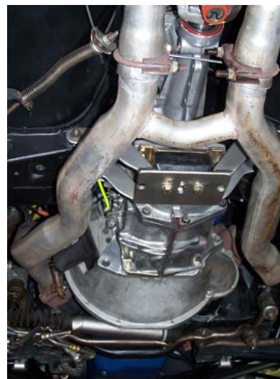
T-5 transmission installed in a '70 BOSS 302
