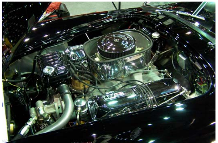
Jim's 427 Sideoiler produces 523.5 HP and 518.8 Lbs-Ft of torque at 5300 RPM's
