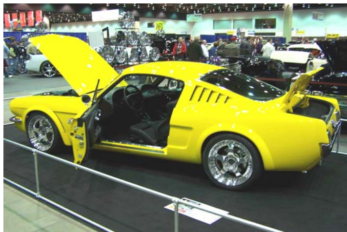
SN65 is a 2003 Mustang chassis, suspension and drive train with a 1965 2+2 body
