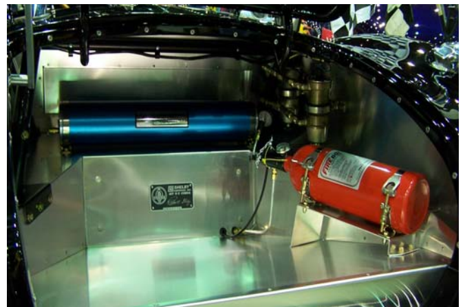
Jim has a fire suppression system and an Accusump located in the trunk of his Shelby 427 Cobra
