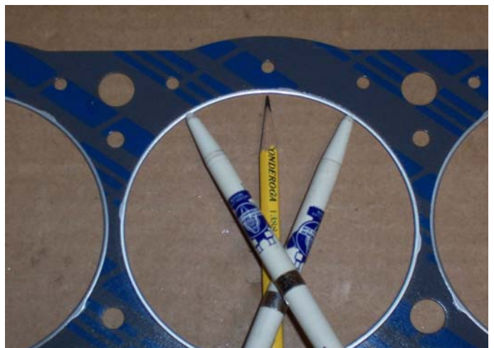
Head gasket holes at the top of the cylinder in the 11, 12 and 1 o'clock positions
