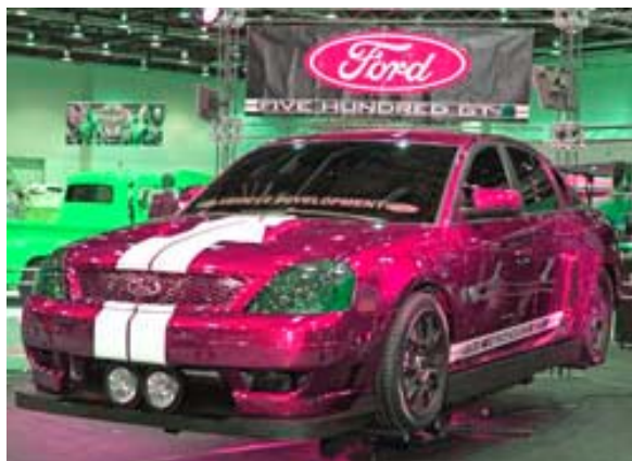
550 HP Five Hundred GT-R uses Ford GT power train and chassis components, wrapped in a Ford 500 body
