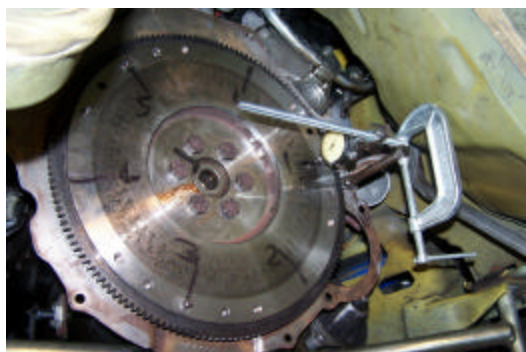
Measuring runout of the flywheel
