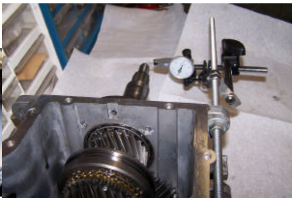
Measuring the transmission input shaft end play
