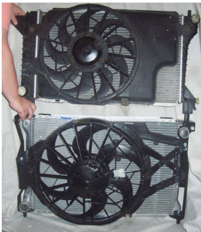
Comparison of original 1996 Cobra radiator and fan assembly (top), vs. 2003 supercharged Cobra (bottom).
