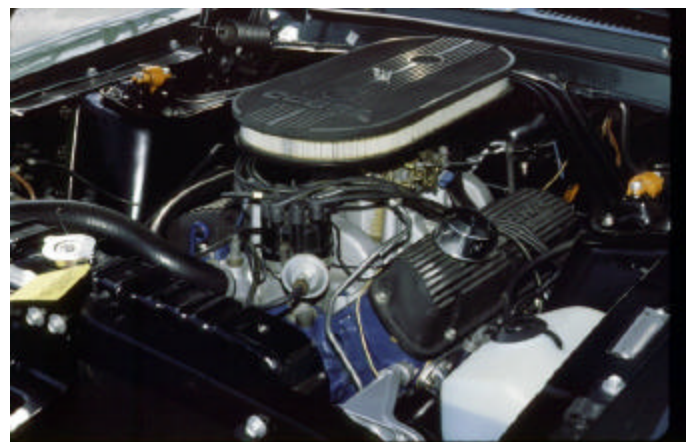
The original 302 V8 was stroked to 347 CI, by Jeff and Walltucky Speed's Jim Murray.
