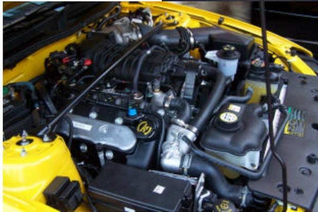
**Shelby Mustang Cobra engine with supercharger**
