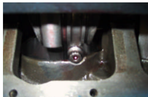
A die grinder was used to make a clearance notch in the bottom of the cylinder bore for the rod bolts
