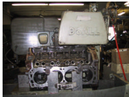
Decking John's block on a DoAll wet grinder
