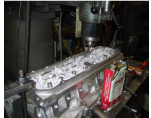
Milling the rocker stud bosses to compensate for the rocker stud hex and guide plate thickness
