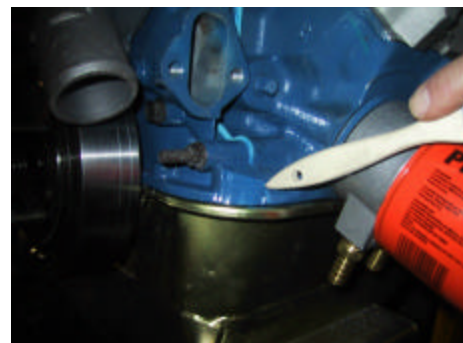
John's front cover with the boss removed to provide clearance for the Edelbrock fuel pump
