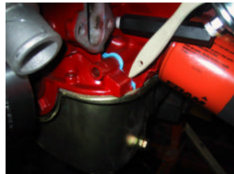
Pat's front cover with the boss below the fuel pump opening
