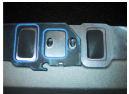
The intake ports were smaller and off center, when compared to the gasket
