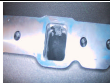
John milled the intake ports to match the gasket
