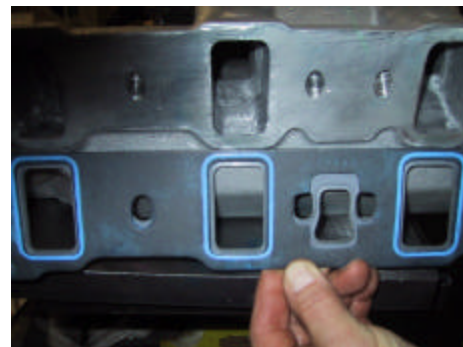
John used a die grinder to blend the milled opening to the rest of the port
