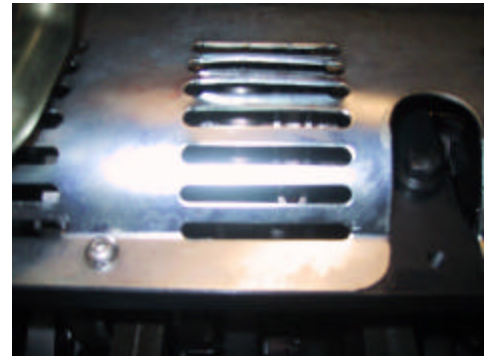
Windage tray tweaked for rod bolt clearance (some louvers had to be bent outward)
