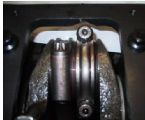
Canton griddle after using a die grinder to make clearance for rod bolts
