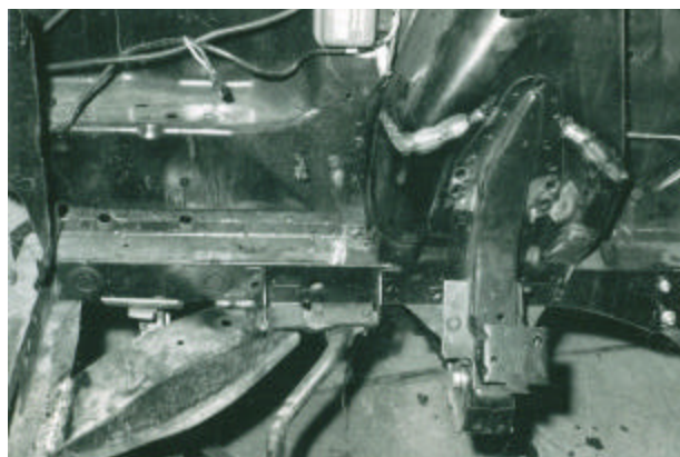
Polaroid picture taken at Kar Kraft in 1970 to document the front structure welding reinforcement as illustrated in Figure 26 of the Chassis Modification book.
