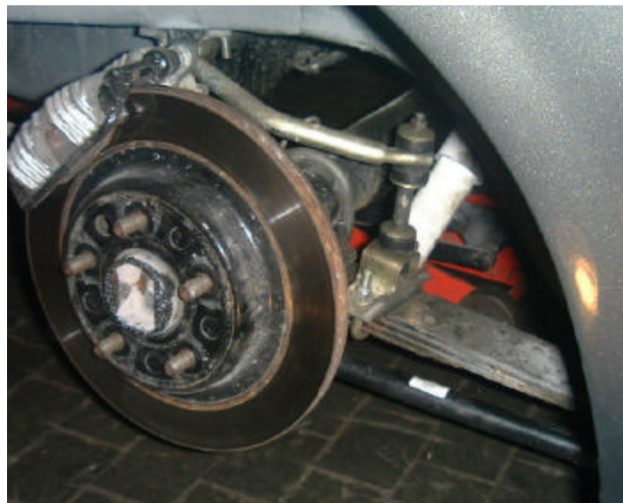
John re-drilled the lug bolt pattern in the 12" Firebird rotor and mounted the PBR calipers via a bracket he fabricated.
