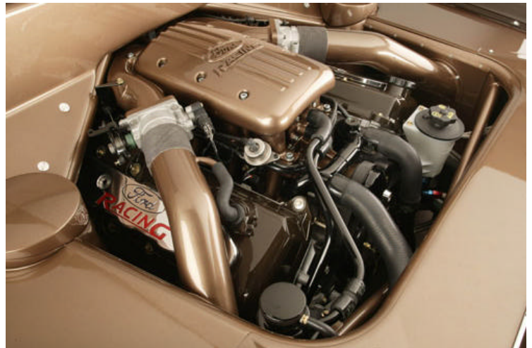
Neat installation of the new 5.0Liter "Cammer" Crate Engine into the FR100 Panel Truck engine compartment.
