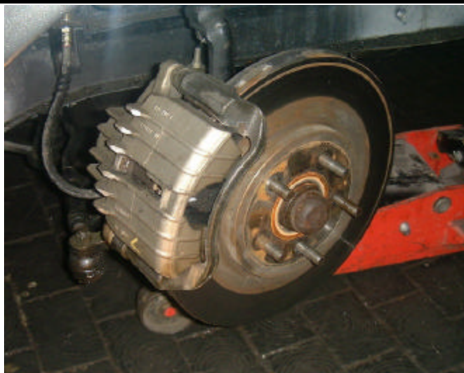
John fabricated a bearing hub to mount the 13" Cobra rotor and a bracket to mount the PBR caliper to convert to front disc brakes.
