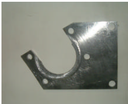
John fabricated a bearing hub to mount the 13" Cobra rotor and a bracket to mount the PBR caliper to convert to front disc brakes.
