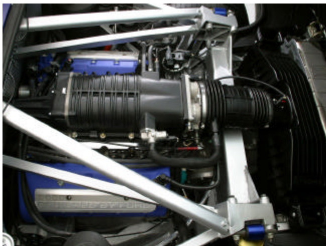
The mid-mounted V-8 breathes supercharged air to deliver 500 horsepower.
