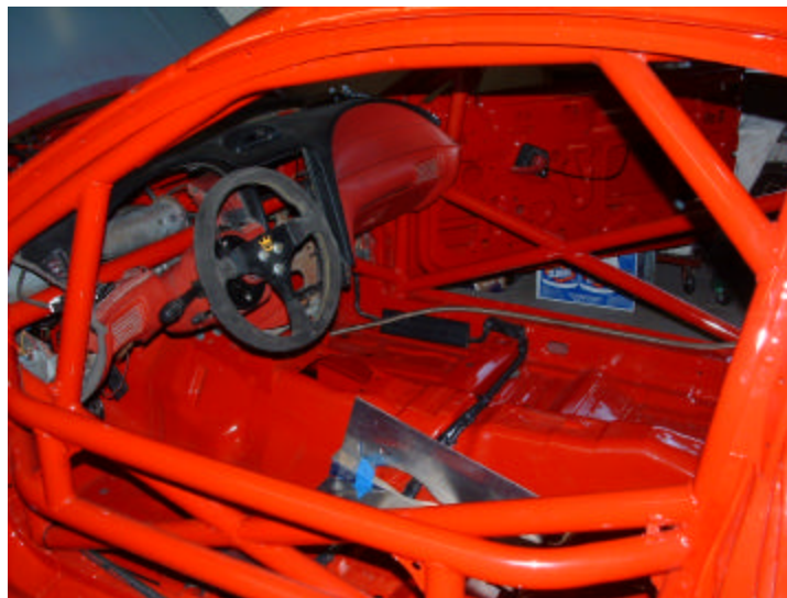
Dash fitted around roll cage. Note the stock steering column with 12" steering wheel.
