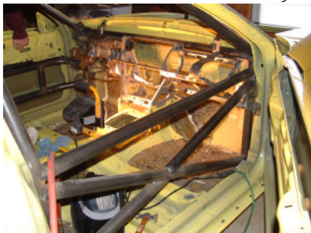
Professionally Designed Roll Cage Installed in the Mach 1 Racer Scott Hoag photo
