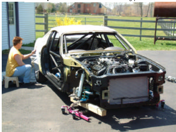
Drivetrain installed in the Mach 1 Racer. Larry Decker is preparing the car for paint. Notice the temporary front suspension. Scott Hoag photo
