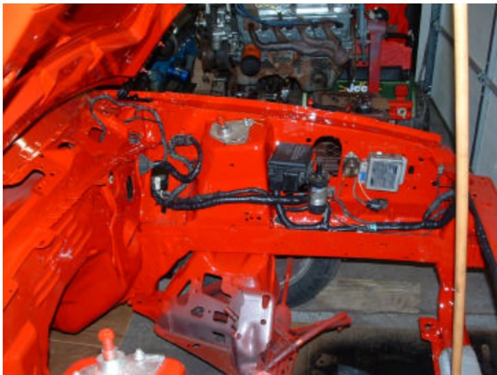
Engine compartment electrical system including Motorsports harness, Dura Spark box with rev limiter and coil
