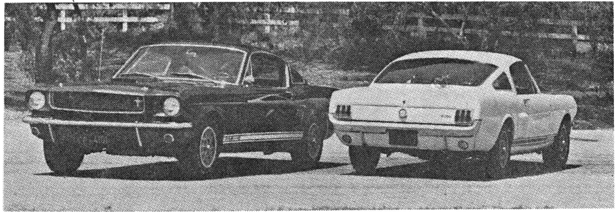
Both cars were fitted with optional cast-aluminum wheels, which enhance appearance and reduce weight but present problems when tire is removed, due to small center.
