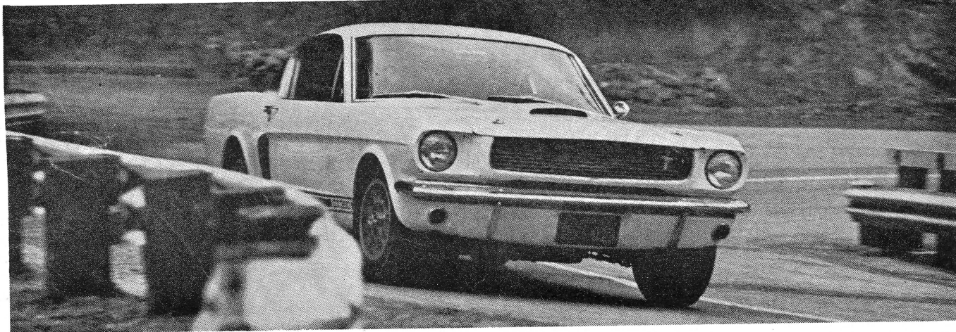
STIFF STEERING MAKES CORNERS NOTICEABLE, AND STANDSTILL TURNS OF THE WHEELS ALL BUT IMPOSSIBLE. OVERALL RATIO IS 19 TO 1.
