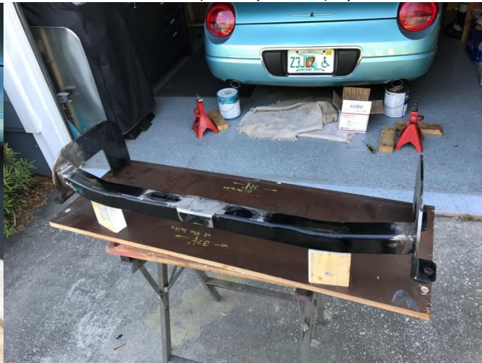
Crossbar relocated UP (in-car position) by ½”
