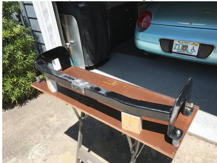
Fixture with bar upside down and ½” gap
